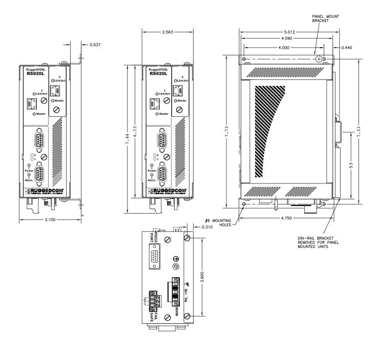
Dual Port Ethernet over VDSL with Integrated Dual Port Serial Device Server, 128-bit Encryption
