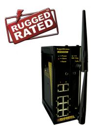
The RuggedWireless™ RS900W is an industrially hardened Ethernet switch which integrates an IEEE 802.11b/g Wireless Access Point, with a fully managed wired 8-Port Ethernet switch providing six Fast Ethernet copper only ports and two optional copper or fiber ports. With the installation of the RS900W wireless access point, a network designer will achieve the integration of wired and wireless networks. The RS900W can be configured as an access, client, or bridge device.
